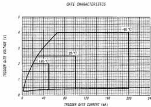
This graph shows required gate current and voltage to trigger all the PGH308 at -40°C, at 25°C and 125°C. For example, we know that DC current of 100mA can turn on every PGH308 at 25°C, and accompanied gate voltage is less than 2.5V.
