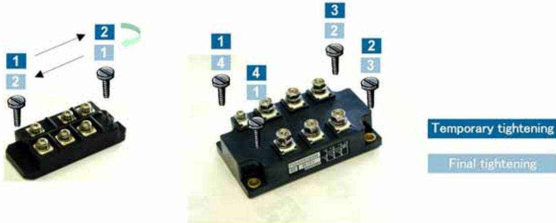
Sequence of tightening screws
