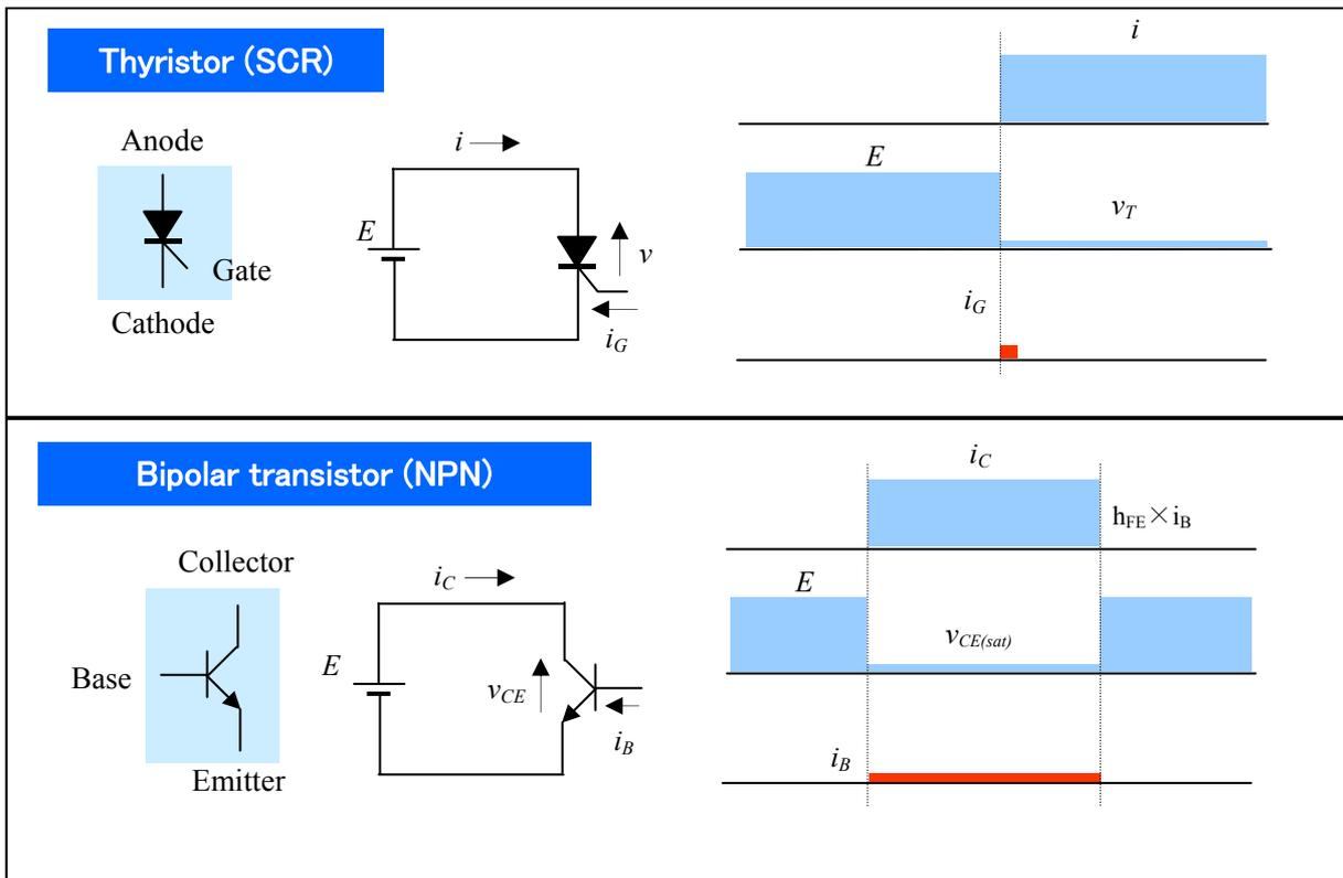
during all of the on-period. At present, major switching devices, such as MOSFET and IGBT, are driven by voltage, but thyristor is current-driven device. Please keep in mind this fact when you design gate firing circuit for thyristor.
