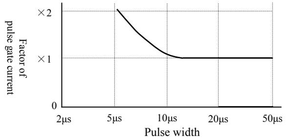
**Typical pulse trigger current**
