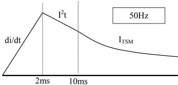
At present, we don't worry whether major power switching devices, such as MOSFET or IGBT, would withstand starting-up current or not even if how fast it is. This is because very small unit-cells are accumulated in one chip, and their high frequency characteristics are remarkably excellent compared with thyristor. By contrast, general thyristor is made of single thyristor unit. Therefore, on-region begins from neighborhood area of gate, and it spreads to the whole chip with time.
